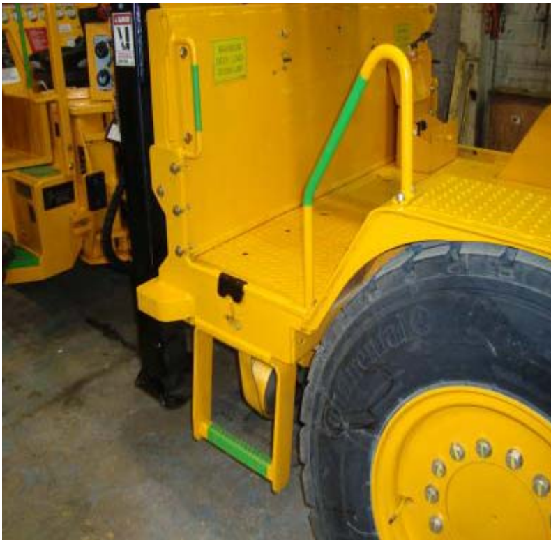
Boom Truck Deck Access
